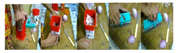
Applying force from top, swivel mechanism and slicing in action
