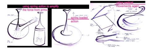
Transforming the vertical force from vertical movement of hands into slicing/chopping (horizontal movement)
