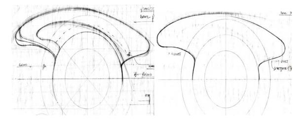
The dimensions of the bowl from top and how/where the blade plate fits in it. Indexing the blade plate with the bowl
