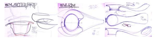
The section of bowl being very important, its edges, how it would be lifted up and how the blade plate fits in it. Also, form development of the handle
