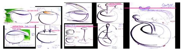
Using vertical force, spring loaded action or swivel mechanisms to amplify the small amount of force
