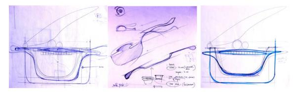
Section of the whole mechanism and how the vegetables/fruits would be pushed down.
