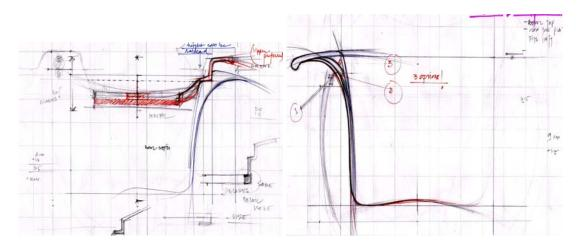
Working out the sections and the details at each point, in all the dimensions and individual components. The bowl in this case, its rim being very important
