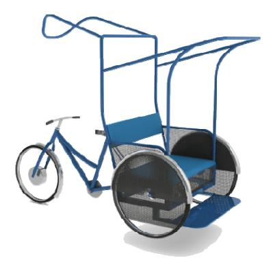
Initial front framing: The frame design was made to minimize material, thereby reducing weight while providing for sufficient strength. The material used was iron as used in the present cycle rickshaws. A triangular frame supports the seat which is connected to the back seating and the two wheels. Then two frames are connected to the triangular frame which tapers at the place which is connected to the handle.
