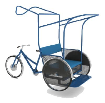
Initial front framing: The frame design was made to minimize material, thereby reducing weight while providing for sufficient strength. The material used was iron as used in the present cycle rickshaws. A triangular frame supports the seat which is connected to the back seating and the two wheels. Then two frames are connected to the triangular frame which tapers at the place which is connected to the handle.
