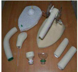
An experimental setup was made up to study the grip parameters. The set up comprised of an iron with an adjustable hinged handle in vertical plane to study effect of handle inclination, an iron with a handle connected to main body with a spherical joint to study azimuthal plane deviations and threaded joints for handles to allow axial rotations and for changing of handles with different curvatures.
