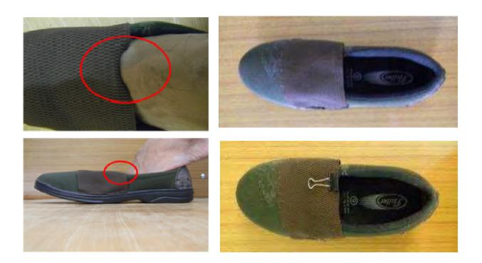
The elastic band open edge finds the steep slope of the foot and cannot follow and rather starts to fold inside.
