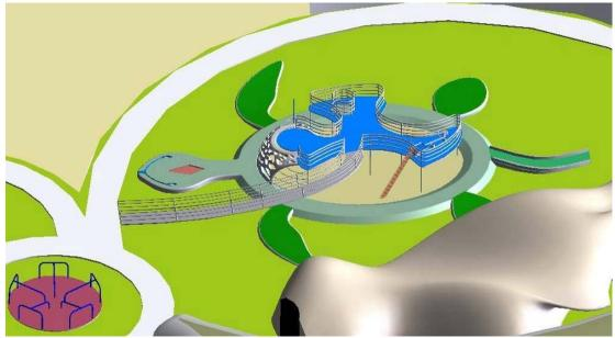
Turtle Tower: An Accessible Play Feature Turtle Tower provides an adventurous and safe environment for all children, with wheelchair access to both the elevated platform and the sand pit. The sand pit serves as a play area, as well as a filtration system for rain water as it passes through to an underground cistern.
