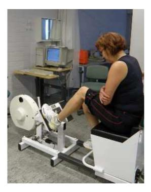
Picture 3. Measuring physical skills: maximum power of lower limb.
