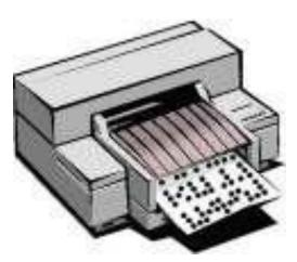
o Braille Embosser - Braille embossers print Braille output from a computer by punching dots onto paper and enable users to make hard copies of documents
