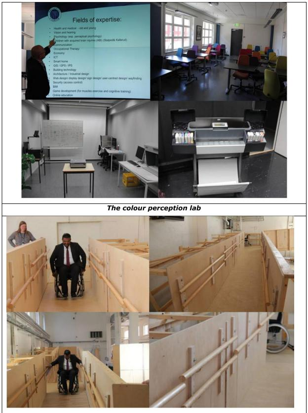
The study of ramps with different gradients, varying surfaces with different materials and varying heights of handrails.
