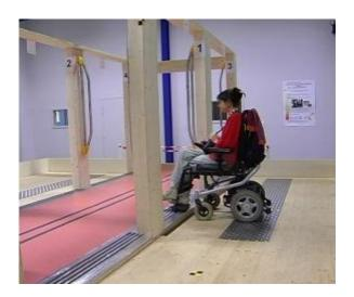
Figure 2: Laboratory tests – level access for wheelchair users (Grange-Faivre, 2013)
