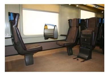
Figure 6: Example of foldable seat, table and hand rest (SNCF, 2009)
