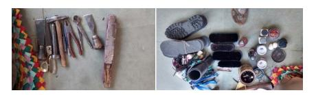
Tools / Materials - Scissor, Hammer, Plier, Chisels, Emery paper on wooden bat, Screwdriver, Iron stand, Needle, Rubber soles, brushes, Adhesive, Laces, oil, nails, nylon thread
