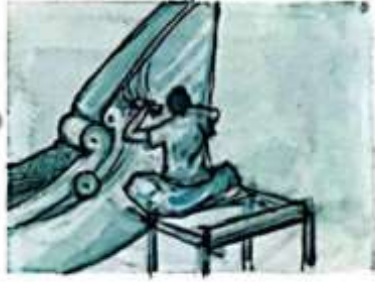
Fig. 9.11 Carpenters carving the Amaram
