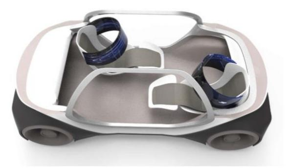
Figure 10: shape memory fabric to smoothen the floor after reconfiguration of interior modules (source: author)
